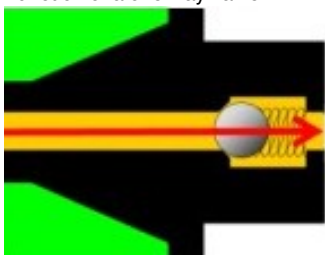
One way valve Spanner Locking ring Rubber gasket One way valve
